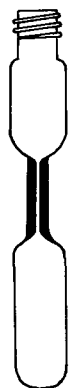
FIG. 1. Apparatus for the preparation of fatty acid methyl esters. Volume of lower bulb is 5 ml, capillary is 3 mm inside diameter and 2.5 cm long, total length of apparatus is 10.5 cm.
